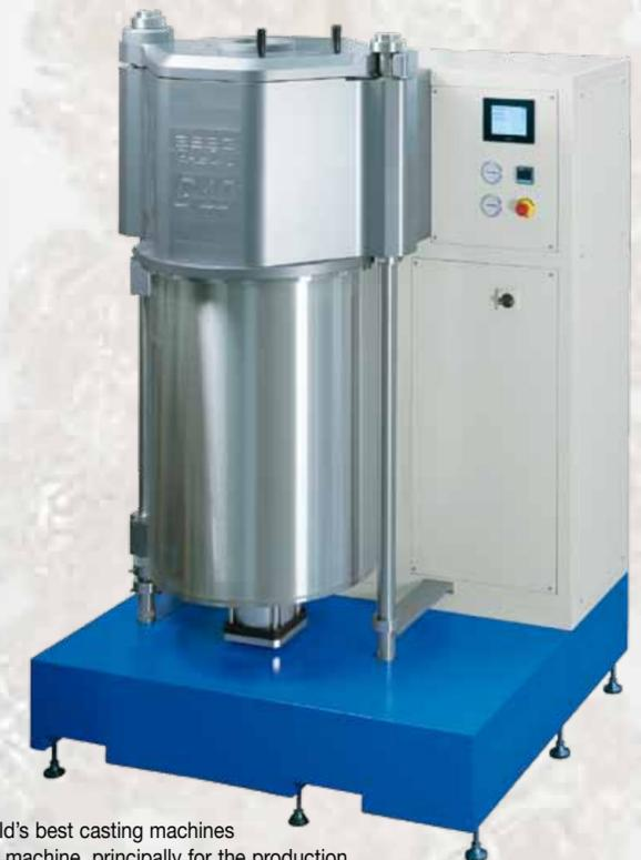
Our "G" series range is currently accepted as the world's best casting machines and we have now introduced the "G10 Heavy - Duty" machine, principally for the production of aluminium castings in the automotive industry, rapid prototyping and various new technologies. It is also capable of producing excellent results in metals such as bronze, brass, silver and gold, etc.
