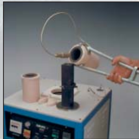
PURE GRAPHITE CRUCIBLE CEMENTED INTO A CERAMIC CONTAINER CAPACITIES 3 AND 6 kg Au CRUCIBLE TONGS WITH GAS BLANKET FACILITY
