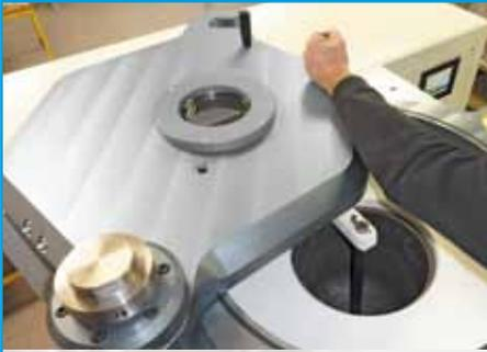
Other machines have tilting covers which have to be lifted for every single cast; this rapidly provokes operator fatigue.
