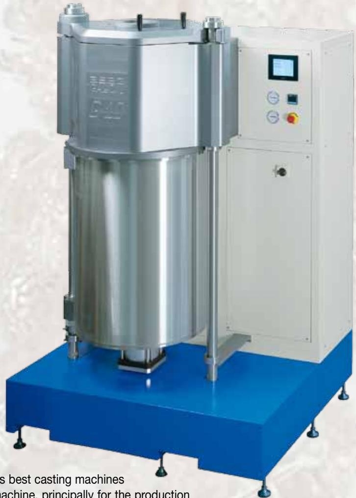
Our “G” series range is currently accepted as the world’s best casting machines and we have now introduced the “G10 Heavy - Duty” machine, principally for the production of aluminium castings in the automotive industry, rapid prototyping and various new technologies. It is also capable of producing excellent results in metals such as bronze, brass, silver and gold, etc.
