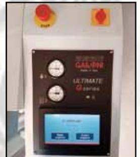
The system used in our "G" series casting machines is a vacuum over-pressure under inert atmosphere. The casting pieces have a very smooth surface, a very dense molecular structure and no defects such as improper filling, porosity and shrinkage.
